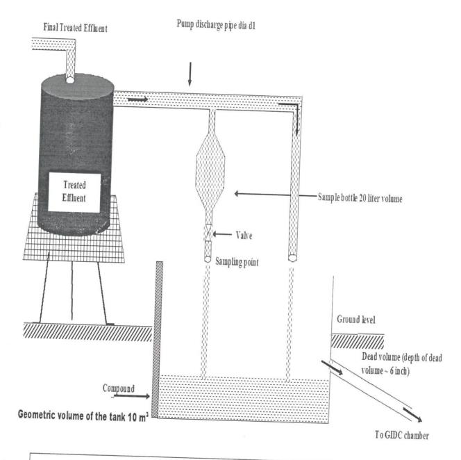
Note d1: Diameter of the discharge line should be such that it can not allow discharging the daily flow in a shorter duration say 2 - 3 hrs. Daily discharge strictly as per CCA, should take at least 18 - 22 hrs a day
